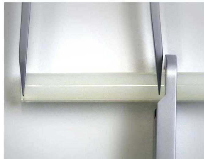
The rod is cut to the desired length using the rod cutting instrument (W01-20)
